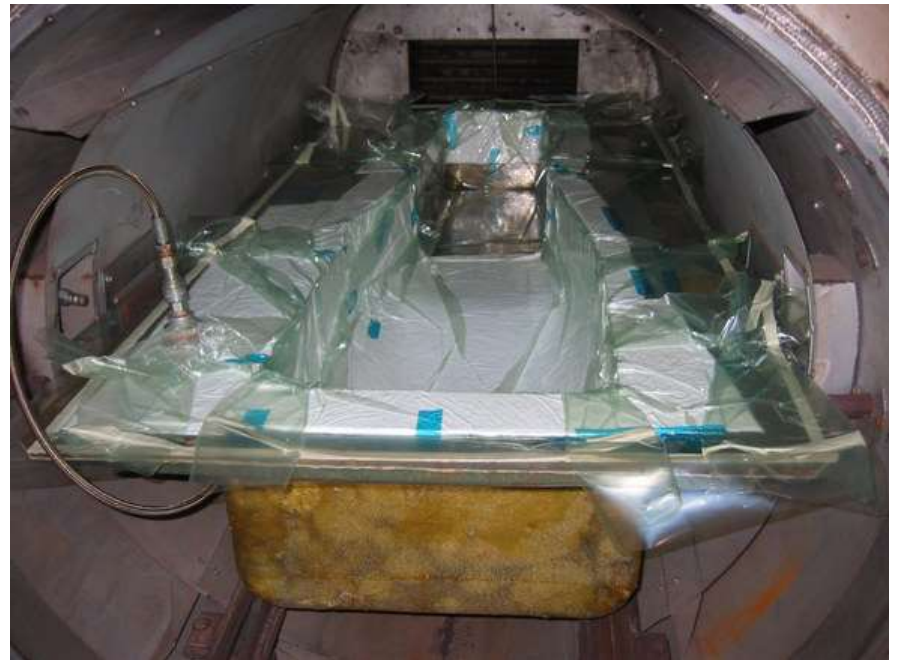
Air being evacuated from bag surrounding mould
