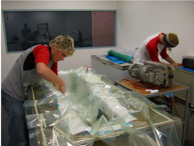
Air bag being applied to mould
